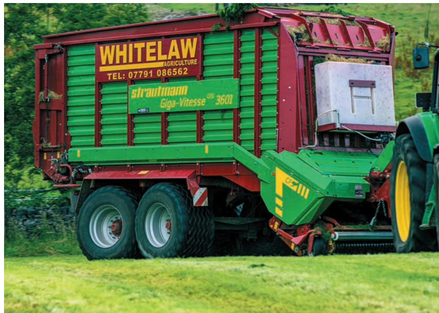
Right: The Giga-Vitesse has a steering axle and the 710 tyres look to be very gentle on the headlands
