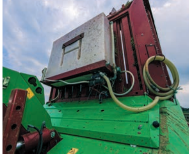
Above: Additive tanks are made from utility van water tanks and look like they were made for the job
