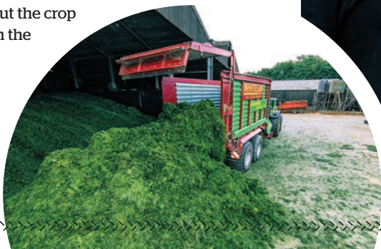
Right inset: Unloading takes about 75 seconds from the bed moving to the tailgate closing
