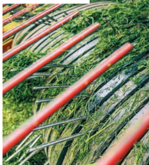
Above: The CFS roller has a flight that spreads the crop out wider and accelerates the grass from the pick-up to the rotor
