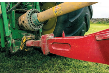
Left: Ball and spoon hitches were adopted after the first season with wagons after excessive wear to hooks and rings
