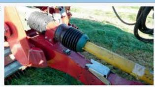
is shaft and gearbox. From the pto, via a protective cam-clutch, this sees power take a 90-degree turn from the front of the machine and sent to the right hand side. From here, a gearbox drives the feed rotor and Continuous Flow System (CFS) roller. Should the gearbox fail, it can usefully be removed
